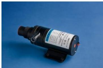
**MACERATOR PUMP:** Toilet waste macerator pump, 20 min. rated, can discharge tanks up to 900 litres.. Cannot run dry! Motor burns
