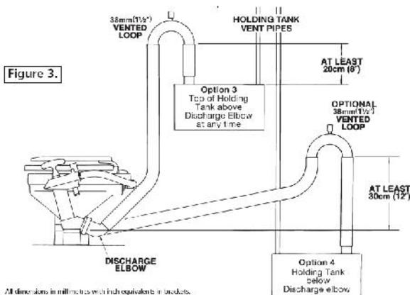
YOU MUST fit a 38mm (1 1/2") Vented loop fitting, MATROMARINE part number 6000100015
