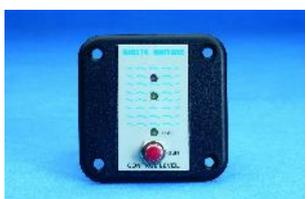
**LEVEL INDICATORS:** Level indicators for clean waters and waste mixture tanks. Probes holder with 5 bushes in which are screwn 5 stainless steel probes for water tanks unit and 3 stainless steel probes for waste mixture tanks unit. Plastic bushes 20 mm long, to avoid risks of short circuit due to humidity inside the tanks. A panel with a scale of 3 leds is advising the almost full tank with a buzzer, for the indicator of waste mixture tanks. Both holders and panels are for VDO connections.
